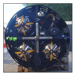
Dimension (LxD1xD2): Weight in Air: Maximum Operating depth: Material: Consumption\* : Autonomy\*: \*Nominal configuration inclu 2.5m x 1m x 0.6m 400Kg (882 lb) 2000m (6,562 ft) Polyethylene, syntactic foam, glass and Titanium < 180mW Up to 4 Years
